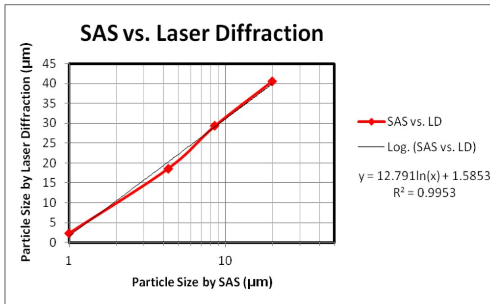
**Figure 7. Comparison of the New Method with Laser Diffraction Particle Size Analysis<sup>10</sup>**
