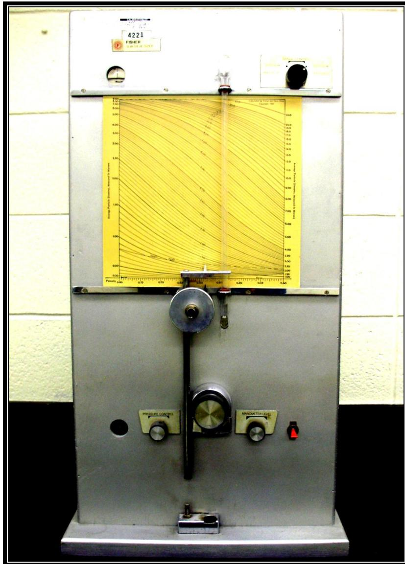
Figure 1. Fisher Sub-Sieve Sizer<sup>3</sup>
