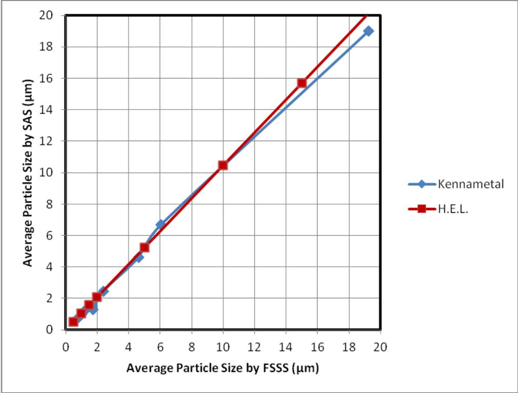
Figure 6. Comparison of Results from Old (FSSS) and New (SAS) Methods<sup>8,9</sup>
