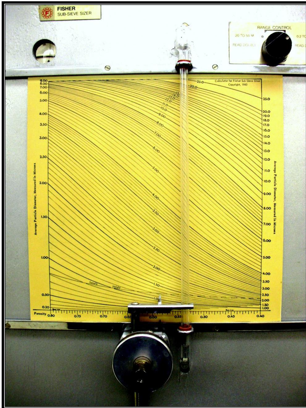
Figure 2. Fisher Sub-Sieve Sizer Particle Size Chart<sup>3</sup>
