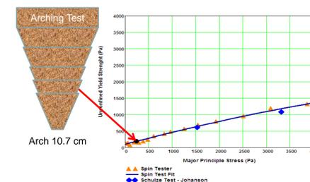
Figure 5. Comparison of the lower stress level unconfined yield strength of Argo corn starch measured with the Schulze direct shear method and the new test technique (SSSpinTester)
