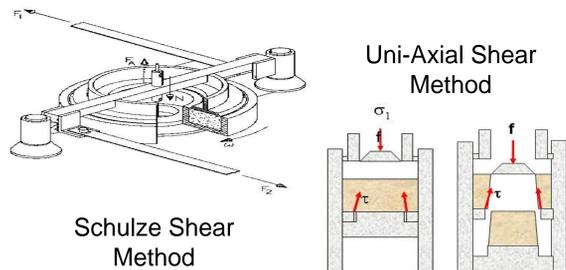
There are several apparatus and methodologies available to measure material bulk strength. Most involve placing a material sample into a test cell, adding compaction pressure and rotating (or shearing) the apparatus until the material fails (falls out of the test cell):
