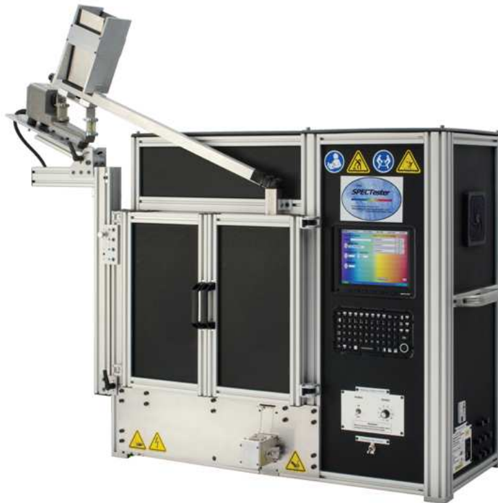
Figure 4. SPECTester used in Segregation Analysis
