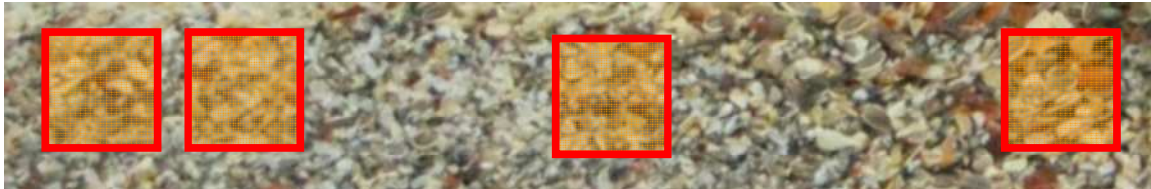
Figure 2. Measurement zone along pile top surface
