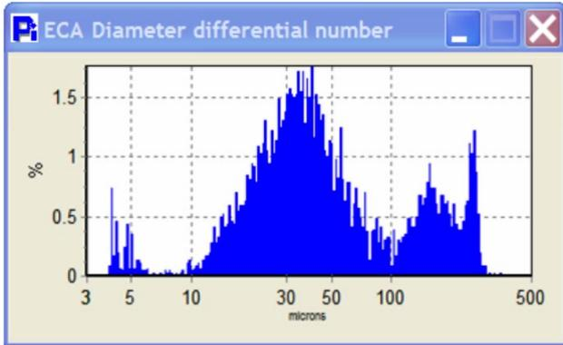
**Figure 3:** Statistical results for flat particles. Note the peaks above 100  $\mu\text{m}$  are the particles that had their largest area oriented toward the viewing point. The particles under 100  $\mu\text{m}$  are variations of particles being analyzed on their other orientations.
