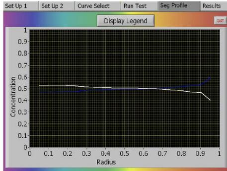
To properly evaluate a material's density using the SPECTester, it is necessary to consider both the Segregation Profile graph as well as the Segregation Intensity Number. Together, these data provide the information necessary to describe the density (or porosity) segregation of a sample mixture.
